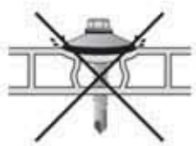
INCORRECT - Excess overtightening
