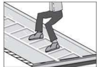
Warning! Do not step on the sheets between the purlins!
