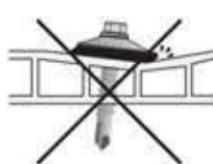
INCORRECT - Non-perpendicular drilling and insertion.
