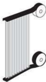
Figure 17b. Installation of Sealing Tape on Open Ends of Sheet
